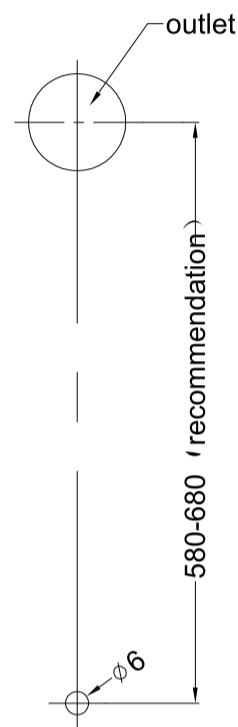
1. Drill a  $\varphi 6$ mm hole at the downwards outlet vertical downward position in the recommendation range.
