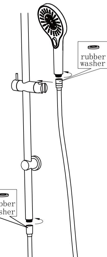
6. Please noted the rubber washer in the hand shower. Connect shower rail and hand shower with hose. TEST & CHECK FOR LEAKS.
