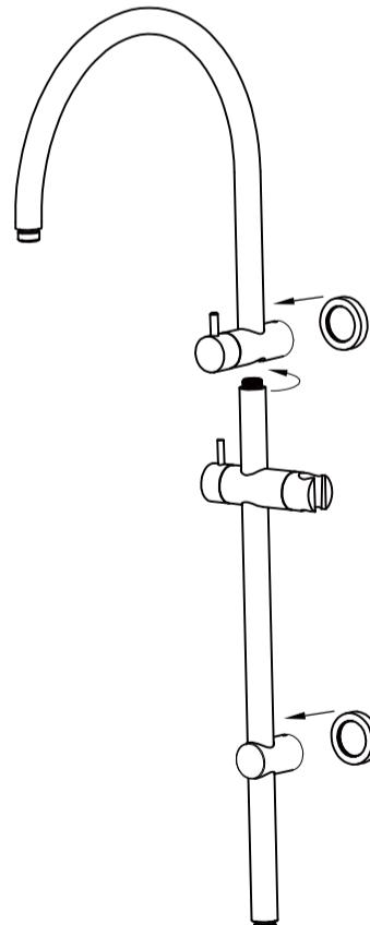
4. Locate and push shower rail assembly onto wall adaptors. Tighten grub screws firmly with allen key provided. Slide the back plates against the wall/tile face properly.
